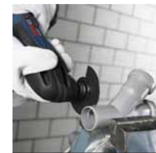
Cutting soft plastics, e.g. trimming of PVC tubes
