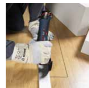
Extremely fine and detailed sawing, e.g. cut-outs in parquet
