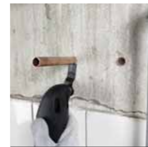
Cutting of non-ferrous metal pieces, e.g. flush cuts of copper tubes
