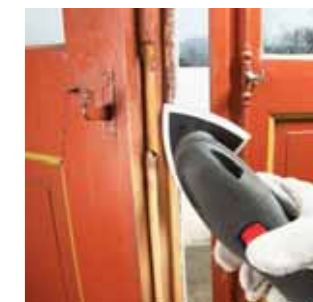
Sanding of fligree and detailed objects, e.g. doors or window frames
