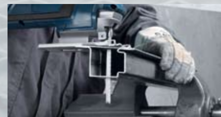
Thin-wall profiles up to 65 mm are easily cut with the T321AF.
